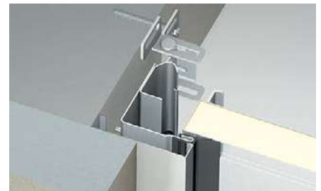
Mounting behind the opening Where side decorative profiles are present
